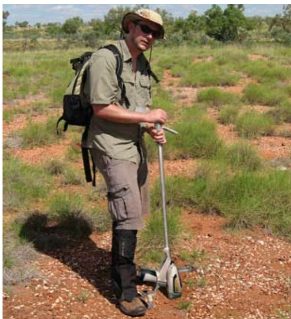
The Thermo Scientific Extend-a-Pole telescoping extension pole and Niton XL3t analyzer with GOLDD technology are the ideal combination for mining and mineral exploration.
