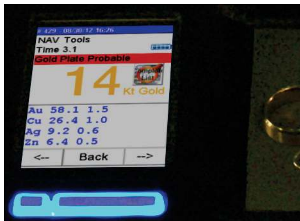
The Niton DXL's patent-pending AuDIT feature instantly warns you of the probability of gold plated material
