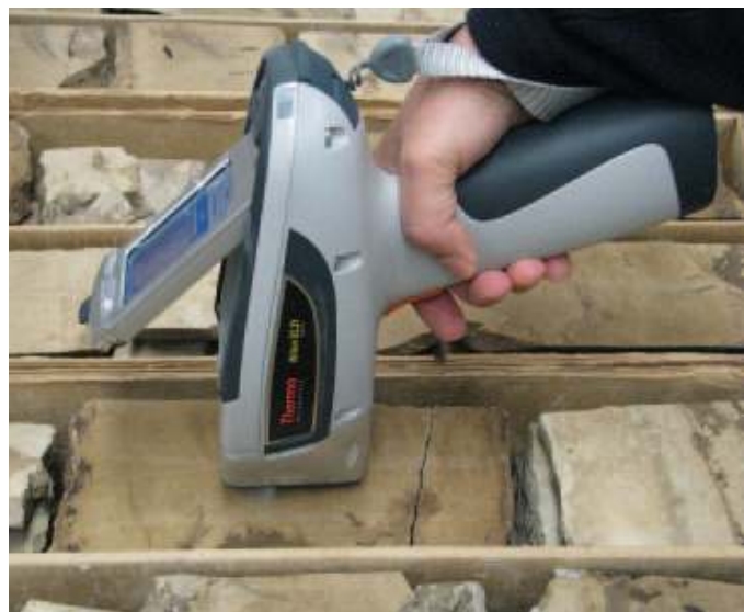
Thermo Scientific Niton XL3t analyzing oil and gas core samples.
